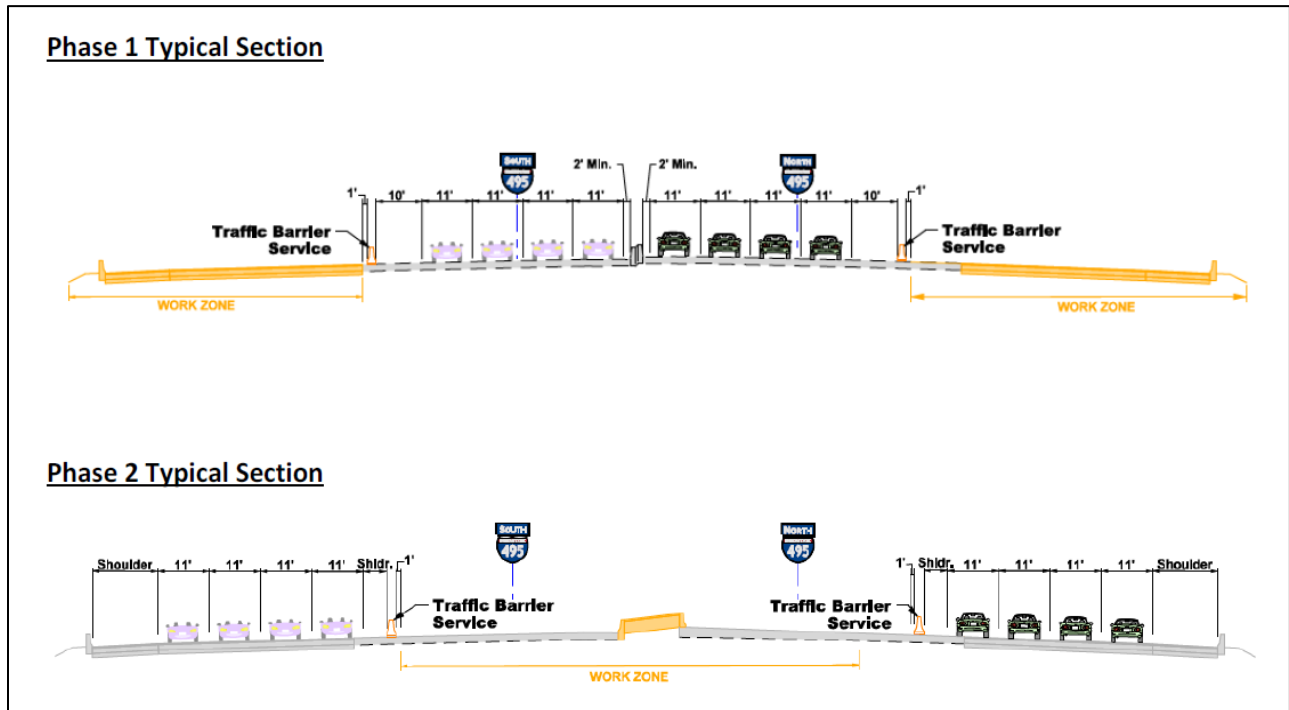
Figure 2.1 Express Lanes and General Purpose Lanes Two Phase Sequence of Construction Typical Section
